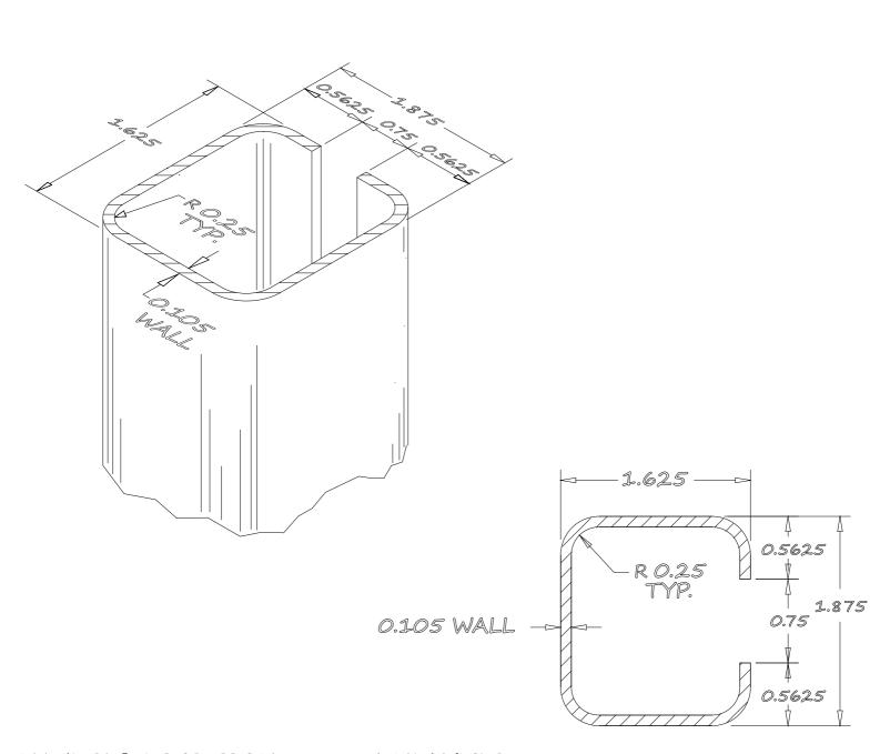
MANUFACTURED FROM 50,000# MIN YIELD STEEL PER ASTM A-570 GRADE 50 AND COATED WITH MINIMUM 20Z ZINC PER SQ. FT PER ASTM F1043-TYPE A (1.85 # PER FT.)
