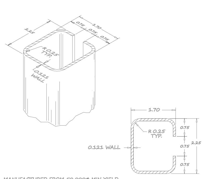
MANUFACTURED FROM 50,000# MIN YIELD STEEL PER ASTM A-570 AND COATED WITH MINIMUM 20Z ZINC PER SQ. FT PER ASTM F1043-TYPE A (2.78 # PER FT.)
