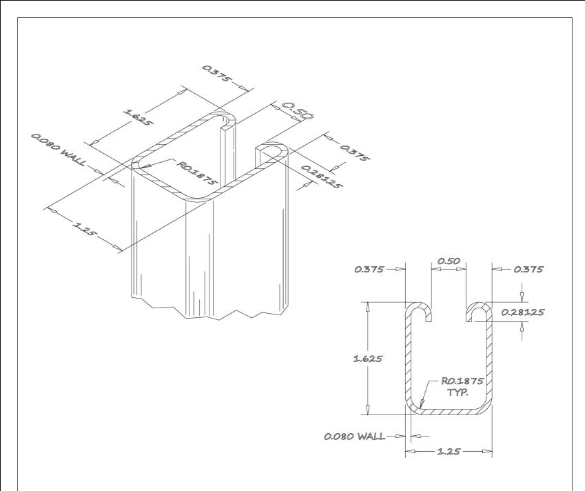
MANUFACTURED FROM 45,000# MIN YIELD STEEL PER ASTM A-570 GRADE 45 AND COATED WITH MINIMUM 20Z ZINC PER SQ. FOOT 2 PER ASTM F1043-TYPE A (1.35 #/FT.)
