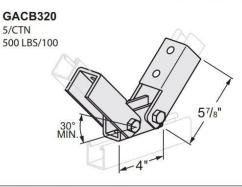
\* MATERIAL IS 1-5/8" WIDE x 1/4" THICK UNLESS SPECIFIED • HOLES ARE 9/16" DIAMETER UNLESS SPECIFIED \*
