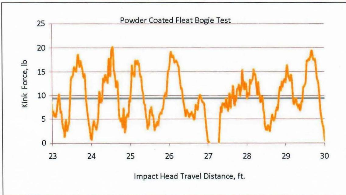
Figure 4. Plot of Kink Force v. Impact Head Travel Distance
