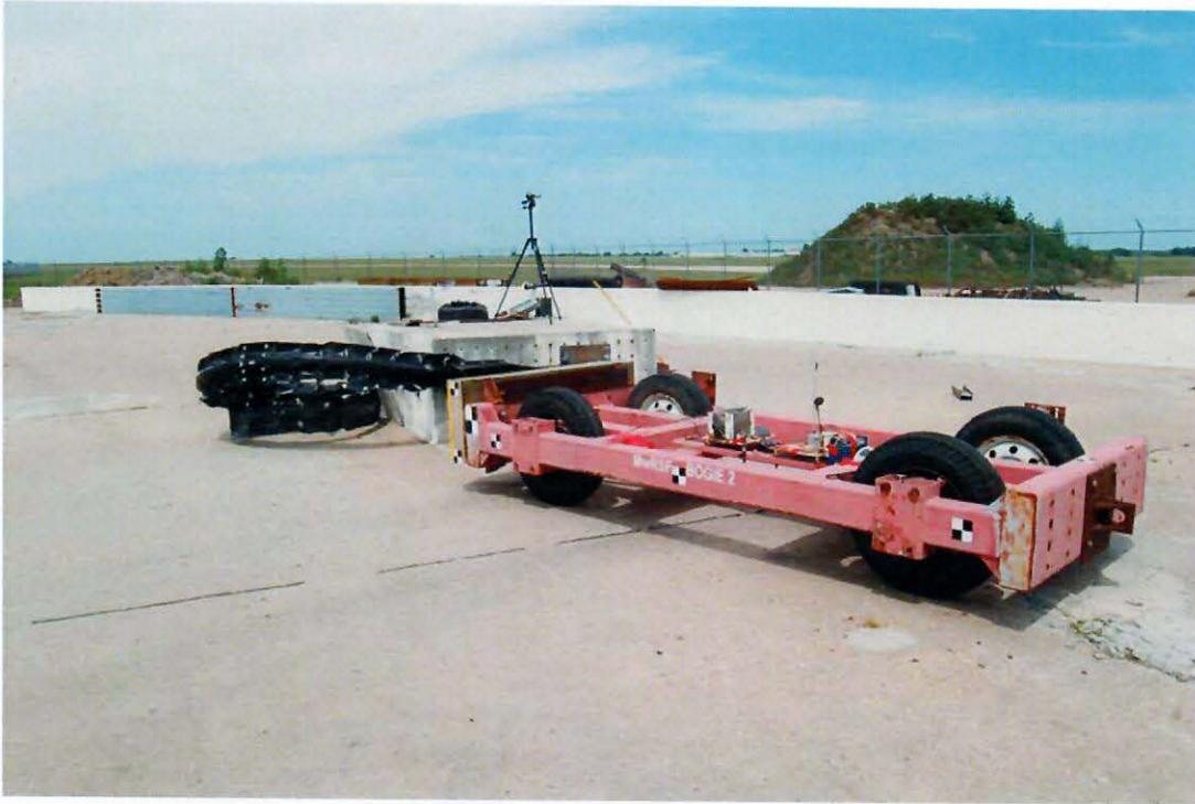
Figure 2. Photographs of Bogie Test Installation After Test
