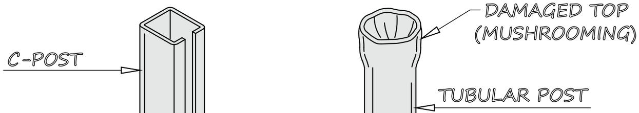
WHEN DRIVING A C-POST, THE DIRT ESCAPES THROUGH THE OPEN CHANNEL RELIEVING THE PRESSURE, WHILE THE BASE OF THE POST WILL ACTUALLY SPREAD ABOUT 1/4" TO 1/2" DUE TO THE UNIQUE 'C' SHAPE.
