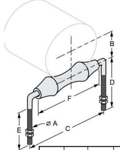
Size Range: 2" through 16" pipe size. Pipe roller size shown is
