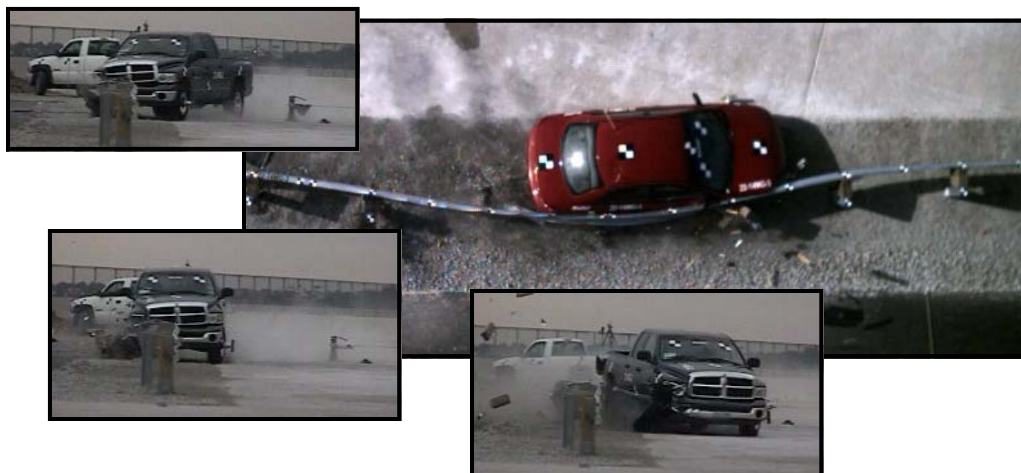
MGS full-scale crash testing with 2270P and 1100C, the proposed NCHRP 350 update vehicles.
